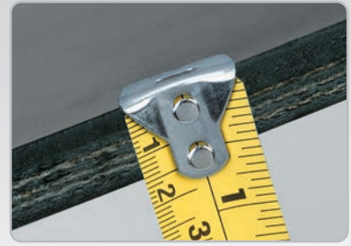
Measure belt thickness.
